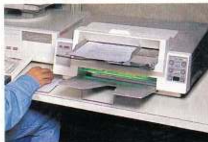
Gobble Gobble The Bell & Howell Copiscan II, which swallowed 150,000 pieces of paper and turned them into computer tape.
